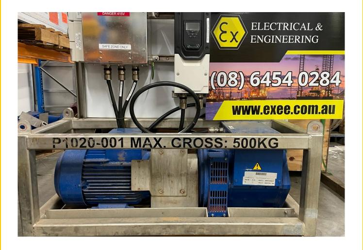
Frequency convertor designed for offshore use and harsh environments. Can take either 50 or 60Hz input and transform it into the desired output.
